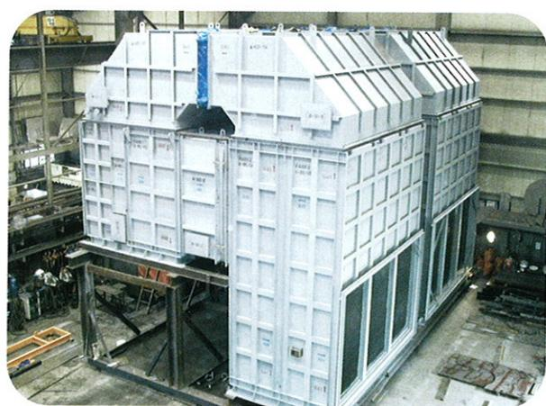
OPEX heat exchanger is optimum and advanced plate type made of smooth and flat plates with the design custom made for each specific application, to ensure;
